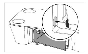
Place the right side door hinge pin into the door frame guide slot. Using a steady force from the top right of the door panel, slide door down until the hinge pin snaps into place.
