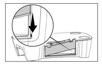
3. Make sure door closes properly and that top retaining pins line up with the top pin sockets.
